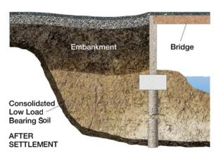
Often poor soil conditions exist at rivers, muskegs or bogs where a bridge structure is supported on a firm foundation either directly or by piles. The road embankment is typically constructed at increased depth due to the ground profile which emphasizes the likelihood of soil settlement when poor soil conditions exist.
